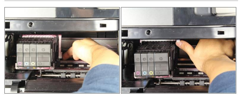
Pull the white plastic tab on the right of the printhead toward you on an upward swing to unlock the printhead.
