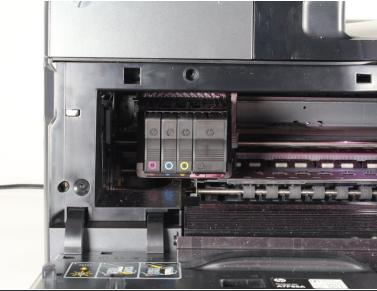
Locate the printer head on the left side of the printer.
