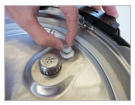
• Pinch the rubber gasket on the float valve and pull up.
