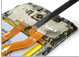
Use the flat end of a spudger to disconnect the display, daughterboard interconnect, and battery cables.
