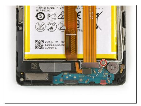
Remove the Phillips #00 screw that holds down the interconnect cable bracket.
