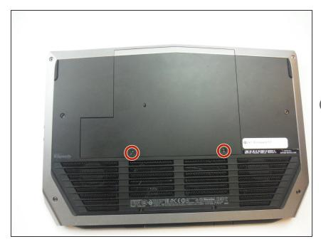
Remove (2) 5 mm Phillips head screws attaching the small access panel to the base using a Phillips # 1 screwdriver.
