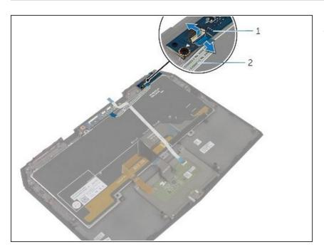
Slide the NEW status-light board cable into the status-light board connector and press down the latch to secure the cable.
