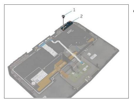
Replace the screw that secures the status-light board to the palm-rest assembly.
