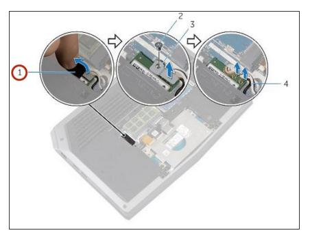
Peel off the adhesive tape from the wireless card.
