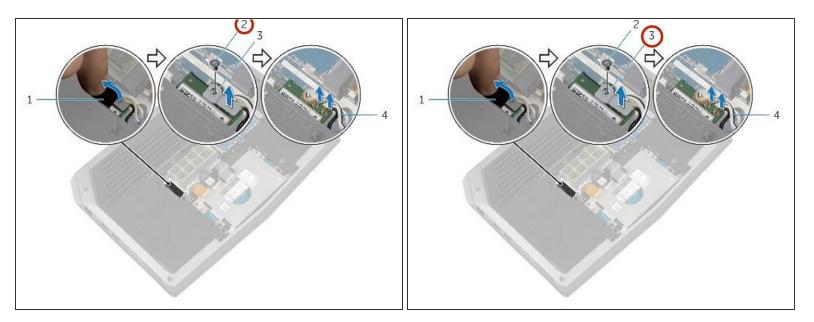
Replace the screw that secures the wireless-card bracket to the wireless card.
