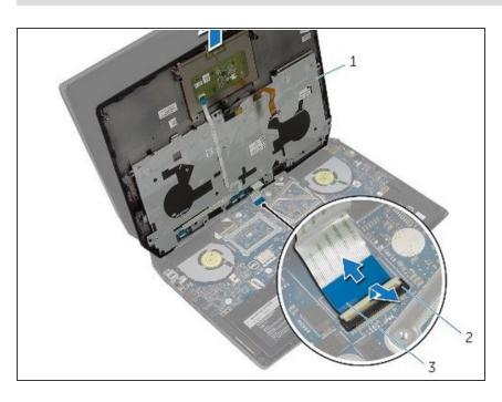
Connect the power-button board cable to the system board.
