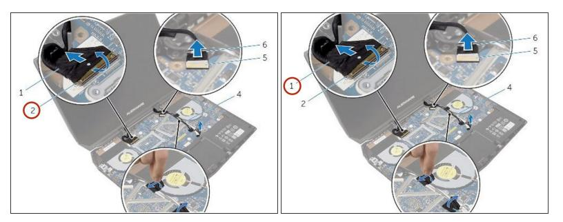
Lift the connector latch and disconnect the display cable from the system board.
