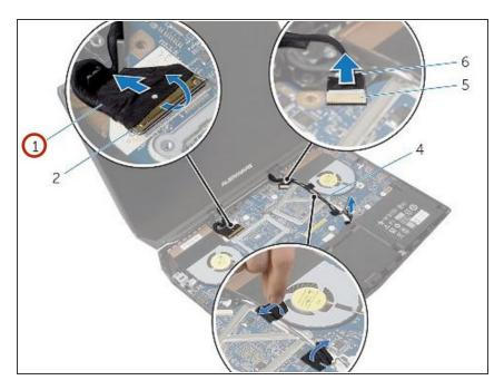
Remove the display cable from the routing guides on the display hinges.
