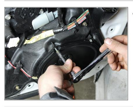
Insert the new speaker and screw into place.
