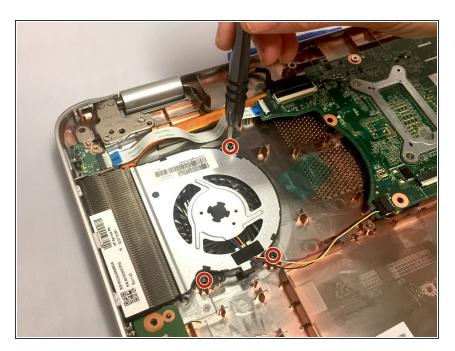
Remove the three 4mm screws using the Phillips #0 screwdriver from the device fan.
