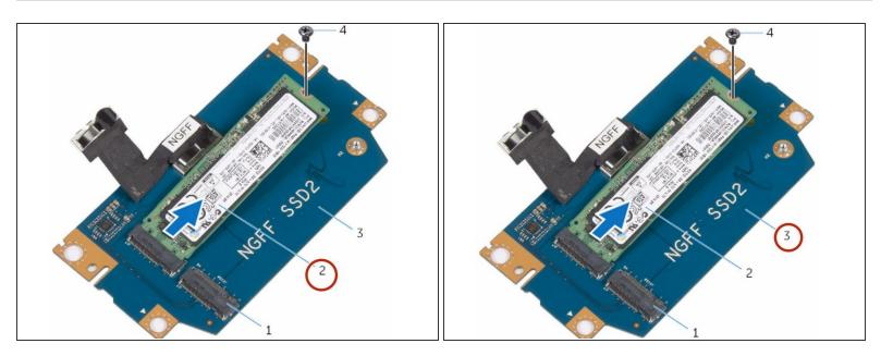
Slide and lift the solid-state drive off the solid-state drive assembly.
