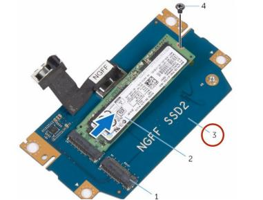
Replace the screw that secures the solid-state drive to the solid-state drive assembly.
