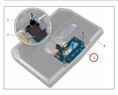
Replace the screws that secure the solid-state drive assembly to the computer base.
