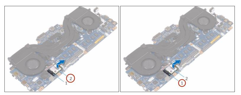
Slide the NEW wireless card into the wireless-card slot on the system board.
