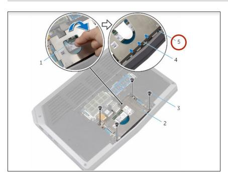
Using the pull tab, disconnect the solid-state drive cable from the system board.
