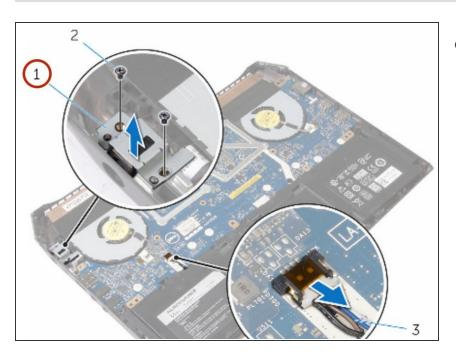
Lift the power-adapter port bracket off the power-adapter port.
