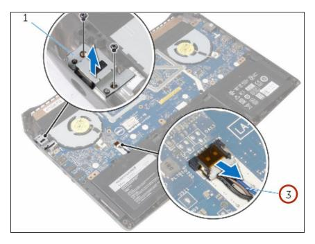
Connect the speaker cable to the connector on the system board.
