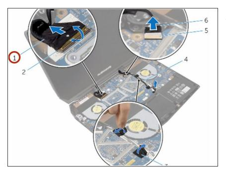
Route the display cable through the routing guides on the display hinge.
