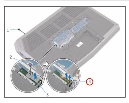
Remove the antenna cables from the routing guides on the display hinges.
