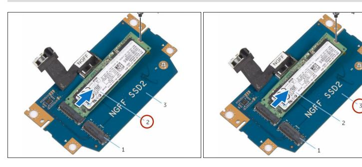
Replace the screws that secure the solid-state drive bracket to the solid-state drive assembly.
