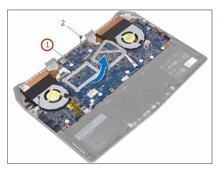
Slide and lift the system-board assembly.
