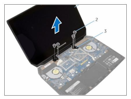
Replace the screws that secure the display hinges to the computer base.
