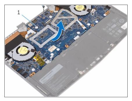
Replace the screws that secure the system board to the computer base.
