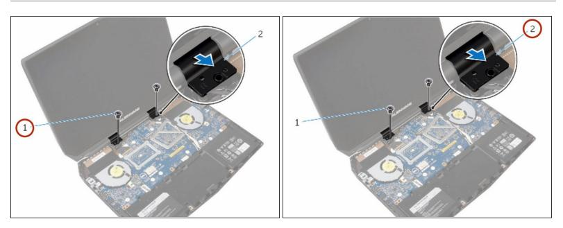
Remove the screws that secure the hinge caps to the display hinges.
