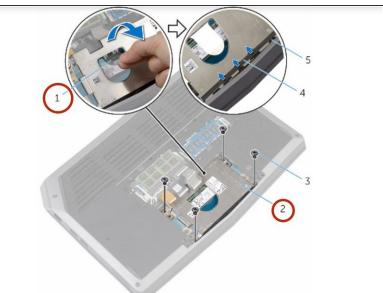
Using the pull tab, pivot the solid-state drive bracket and peel off the bracket from the tabs on the computer base.
