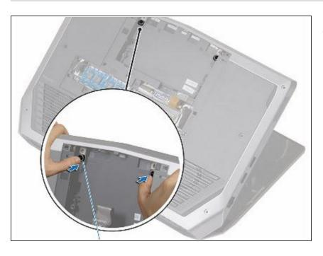
Lift the computer base slightly and push the release tabs on the palmrest assembly until it pops out.
