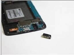
• Insert your finger nail into the groove under the Auxiliary Port and pry the Auxiliary Port out.
