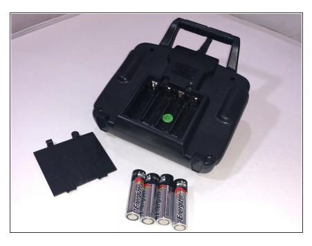
Remove all of four of the AA batteries from the controller. To reassemble your device, follow these instructions in reverse order.
