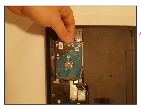
• Lift hard drive out of the computer slightly.
