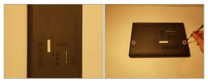
• Use a JIS #0 screwdriver to unscrew the two 6 mm screws from the back panel.
