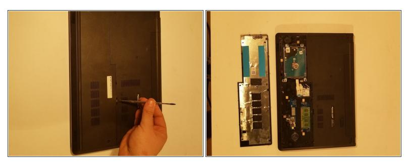
• Using a spudger, lightly lift the RAM cover up and at an angle, away from the computer.
