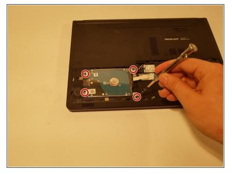
• Remove the four 6 mm JIS #0 screws from the hard drive.
