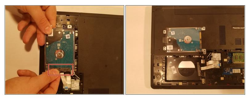
• Using two fingers, grab the black connector on the ribbon, and pull until detached.
