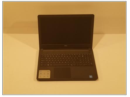
• Make sure the laptop is powered down before you remove the battery.
