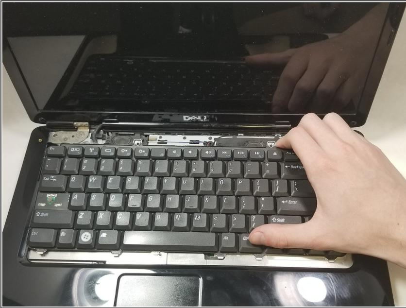
**⚠** Be careful when pulling the keyboard away from the laptop, you may damage the connector holding it to the motherboard.
