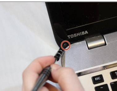
Open the laptop and unscrew each of the screws that are in the corners of the screen using a Phillips #1 screwdriver.
