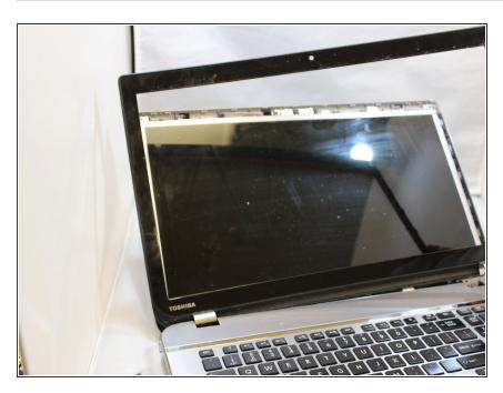
Remove the frame from the device.
