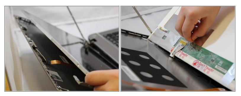
Disconnect the webcam from the screen and unhook any tape.
