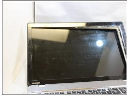
Using a metal spudger, insert the spudger around the edges and the bottom to detach the frame from the screen.
