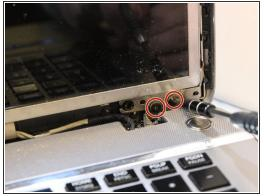
Using a Phillips #1 screwdriver, unscrew all of the screws on the sides of the screen.
