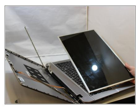
Remove the display from the device and add the new one.
