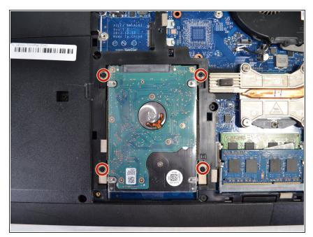
Remove the four 1.2mm Phillips #0 screws from the hard drive.
