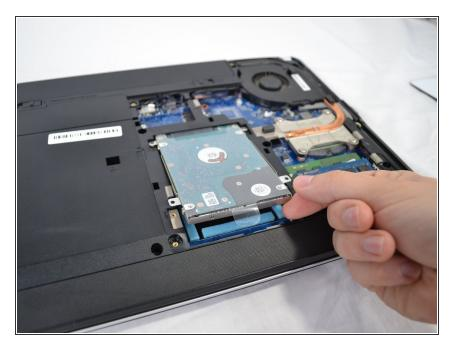
Pull up on the hard drive to allow for removal.
