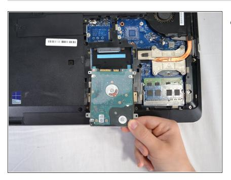
Disconnect the hard drive and pull out to remove.
