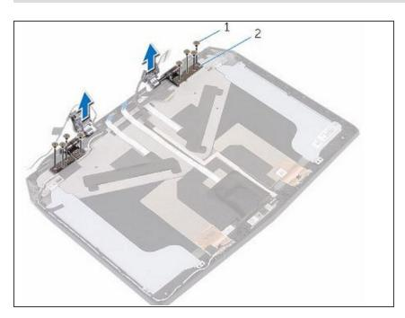
Align the screw holes on the NEW display hinges with the screw holes on the display back-cover.
