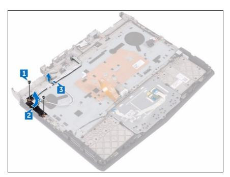
Align the screw holes on the powerbutton board with the screw holes on the palm-rest assembly.
