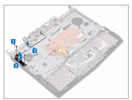
• Lift the power-button board, along with its cable, off the palm-rest assembly.
