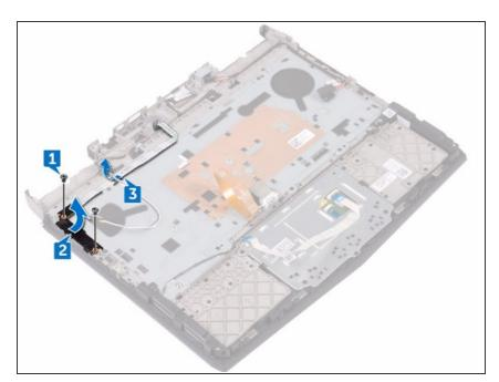
• Using the alignment posts, place the **NEW** power-button board on the palm-rest assembly.
