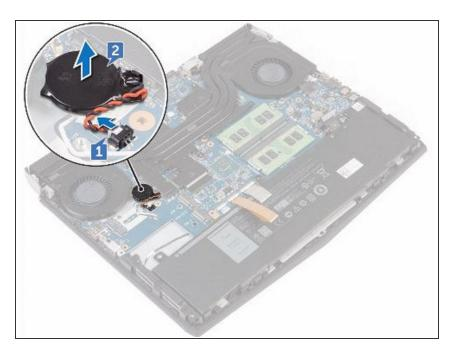
• Adhere the **NEW** coin-cell battery to the palm-rest assembly.
