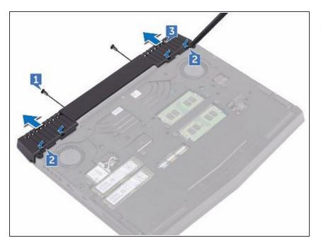
Slide the NEW rear-I/O cover into the slots on the computer base and snap the rear-I/O cover into place.
