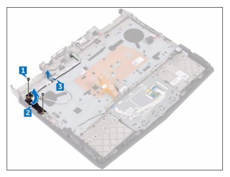
Replace the two screws (M2x3) that secure the power-button board to the palm-rest assembly.
