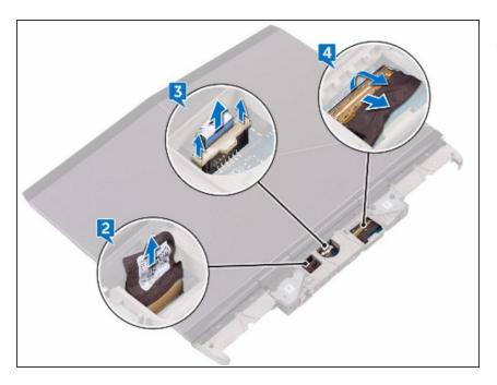
• Open the latch and disconnect the display cable from the system board.
