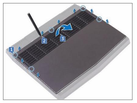
Slide the tabs on the NEW base cover into the slots on the computer base and snap the base cover into place
