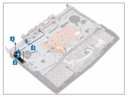
• Adhere the power-button board cable to the palm-rest assembly.
