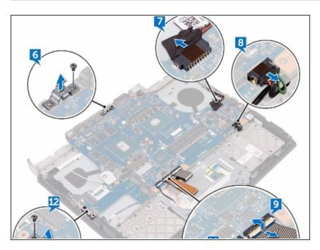
• Slide the keyboard cable into the connector on the system board and close the latch to secure the cable.
