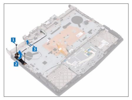
• Peel the power-button board cable from the palm-rest assembly.
