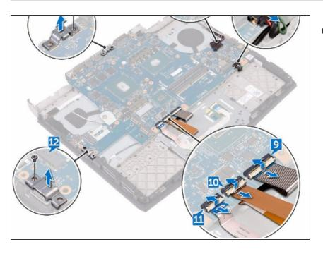
Remove the two screws (M2.5x6L) that secure the system board to the palm- rest assembly.
