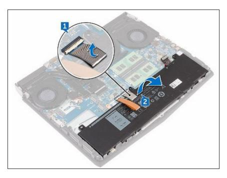
Lift the battery off the palm-rest assembly.
