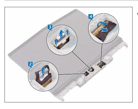
Using the pull-tab, disconnect the power-button board cable from the system board.
