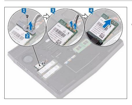
Lift the wireless-card bracket off the wireless card.
