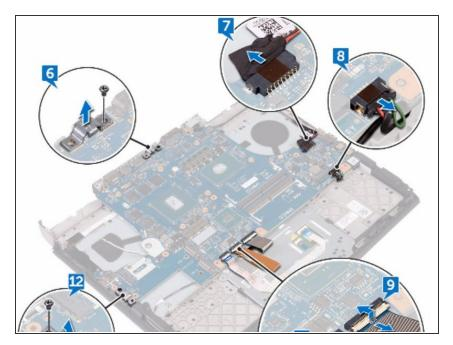
Open the latch and disconnect the keyboard-backlight cable from the system board.
