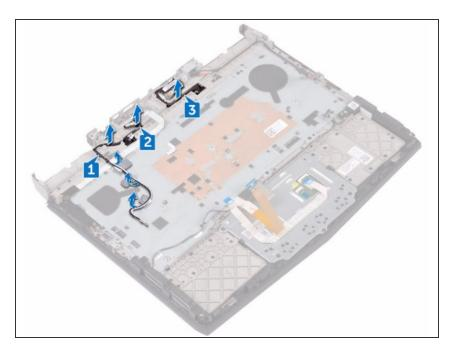
Remove the logo-board cable from the routing guides on the palm-rest assembly.
