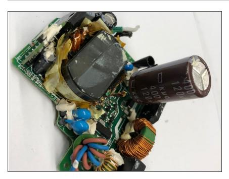
The large capacitor on the circuit board can be bent upright to show more components underneath it.
