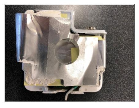
One part of the outer casing (referred to as the top part of the case) is removed revealing an aluminum wrapping.
