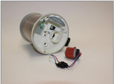
• Remove the electromotor by hand.
