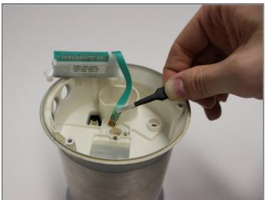
• Pull out the green ribbon cable through the rubber cover.
