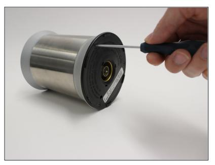
Remove the 12mm Torx screws (x3) from the bottom of the foamer using a Torx TR10 screwdriver.
