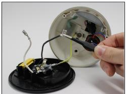
• Take out the grey and white power cables by pulling out the slide connectors from the base.
