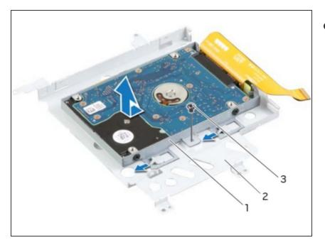
Turn the secondary hard-drive assembly over.
