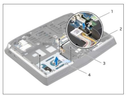
• Align the screw holes on the primary hard-drive assembly with the screw holes on the computer base.
