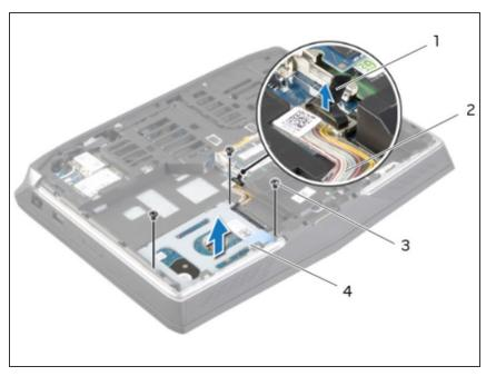
• Connect the primary hard-drive cable to the system-board connector.
