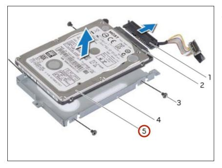
• Slide and lift the primary hard-drive off the primary hard-drive bracket.
