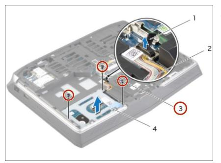
Remove the screws that secure the primary hard-drive assembly to the computer base.
