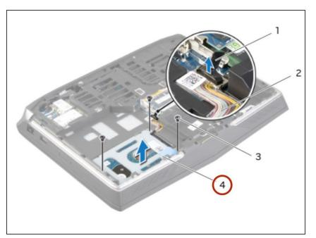
• Lift the primary hard-drive assembly off the computer base.
