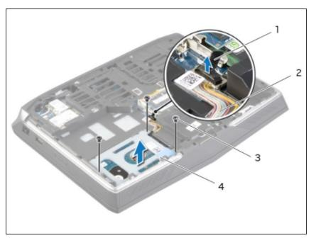
• Replace the screws that secure the primary hard-drive to the primary hard-drive bracket.
