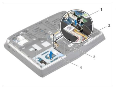
Replace the screws that secure the primary hard-drive assembly to the computer base.
