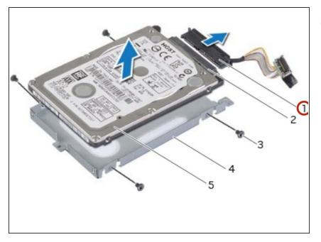
• Disconnect the interposer from the primary hard-drive connector.
