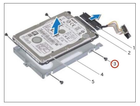
Align the screw holes on the primary hard-drive with the screw holes on the primary hard-drive bracket.
