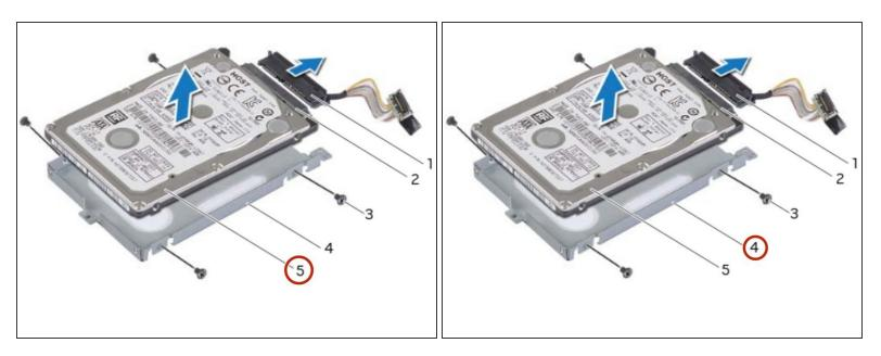
• Slide the **NEW** primary hard-drive into the primary hard-drive bracket.
