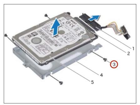
• Remove the screws that secure the primary hard-drive to the primary hard-drive bracket.
