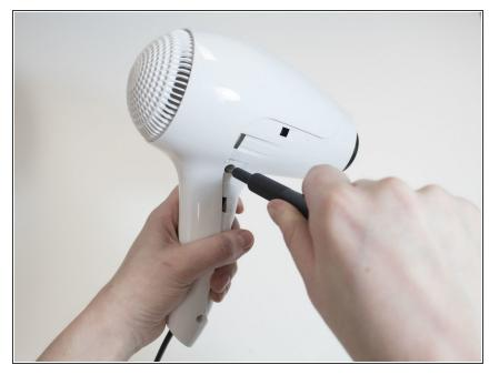
Using the same driver as before, remove the 1.5mm Spanner 4.0 screw that becomes accessible after removal of the front cap.
