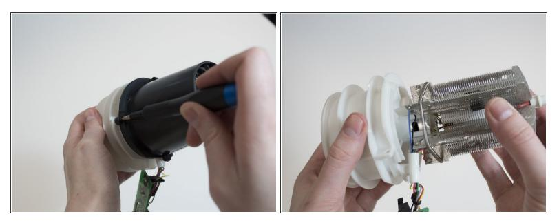
Separate the black inner casing from the other parts by removing the three 1.4mm Phillips #1 screws with a <u>Phillips #1 screwdriver or bit</u> and sliding it off.
