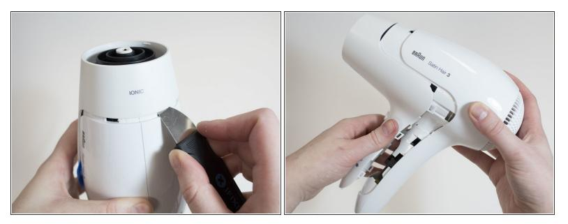
• After opening the last snap-fit of the front cap, it comes loose from the external case halves. Slide the front cap off the external casing and put it aside.
