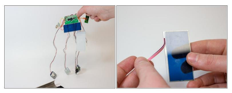
• Lift out the complete electronic circuit and remove the screen and connector.
