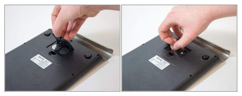
• Remove the battery cover and batteries.
