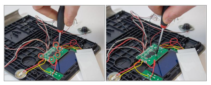
Unscrew the 5 screws from the PCB and screen (round cross head 1,5 mm; 6 mm).
