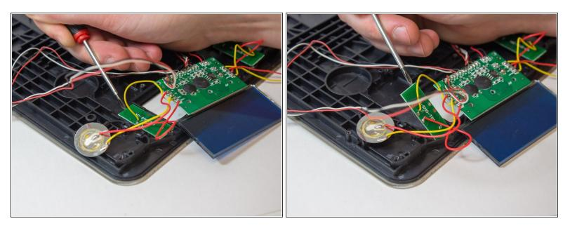
• Pry out the PCBs which include the touch sensors (2).
