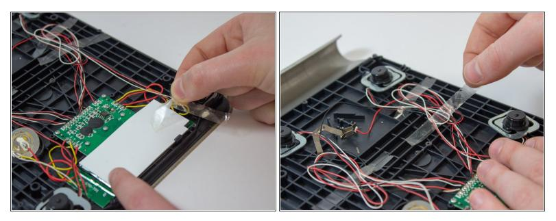
• Remove the tape which holds the electrical wires in place.
