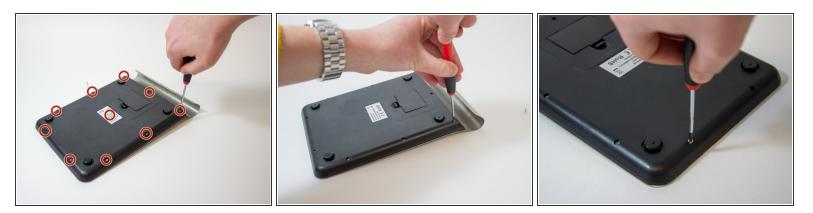
• Unscrew the ten screws (countersunk cross head 1,5 mm; 8 mm).
