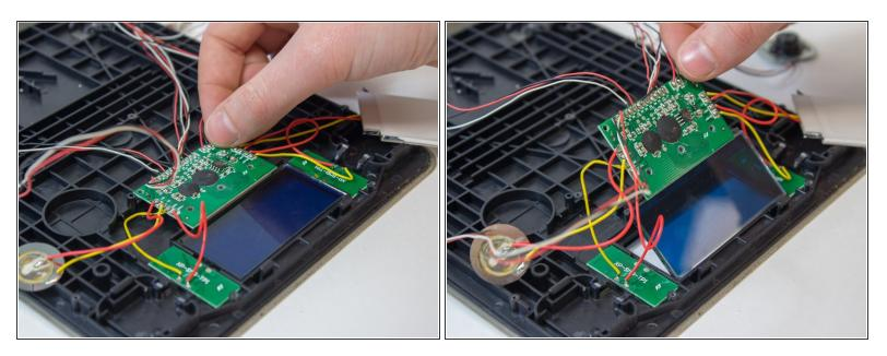
• Lift out the PCB and screen.
