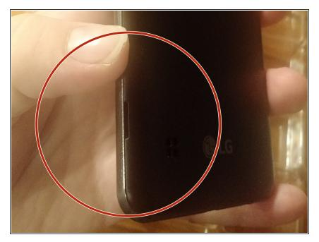
Gently pry open back cover starting at the tab opening and gently working along the perimeter of the phone
