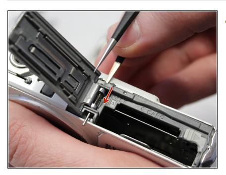
Push the metal bar down using the metal tweezers.
