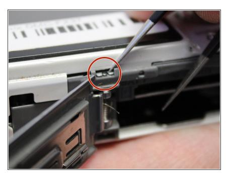
At the left hand side, locate the head of the metal bar that holds the spring in place.
