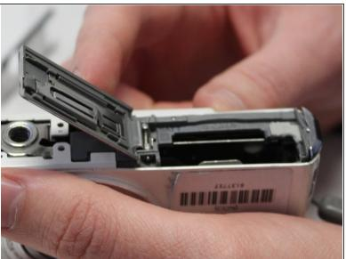
Set the switch on the battery door to "open," and open the door.
