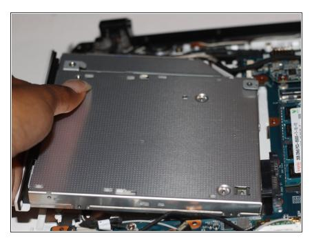
With your hand, grasp the side of the DVD/CD drive and gently pull it out of the socket, disconnecting it from the motherboard.
