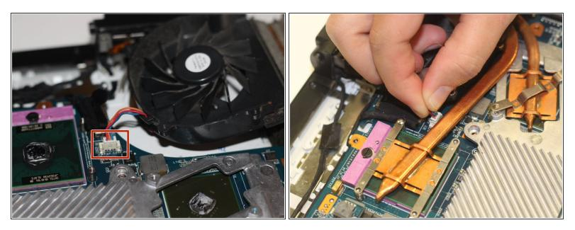
Using your fingers, grasp the white tab and firmly, yet gently, pull up on the wire to disconnect it from the motherboard.
