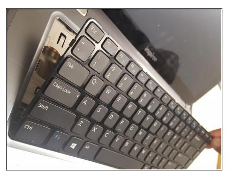
Using a nylon spudger, push the retaining clips away from the keyboard - there are five along the top row, and two on each side. You can carefully pull the keyboard away from each clip when it's released. The bottom edge of the keyboard will just pull away.
