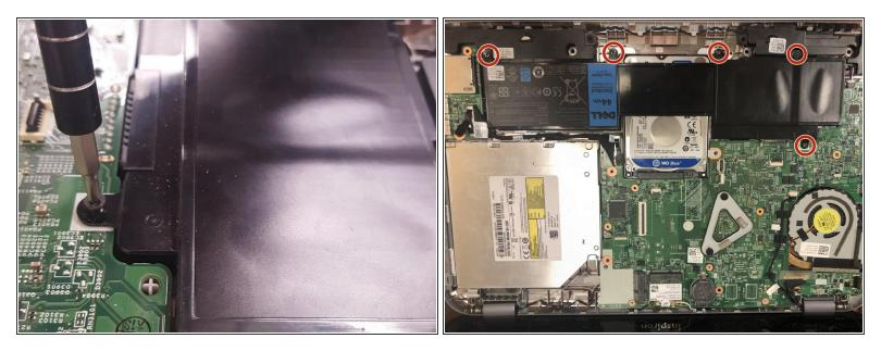
• Take the battery out by unscrewing the 5 screws and pulling straight off.
