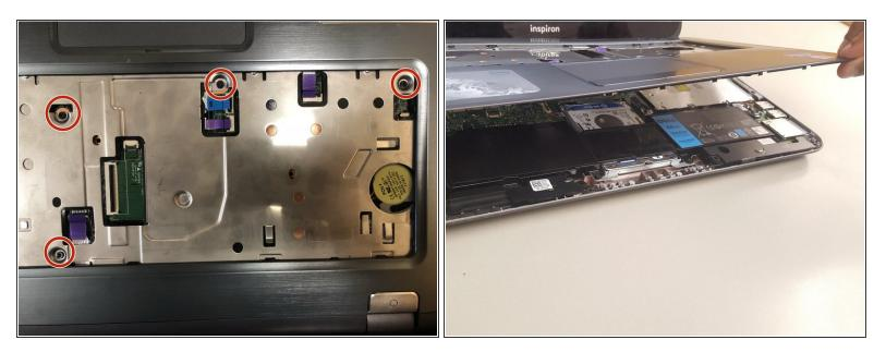
Unscrew the surface under the keyboard and remove top plate from the base.
