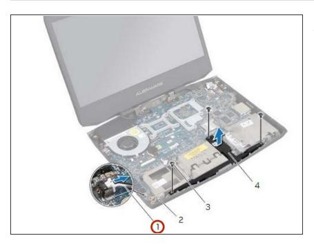
Disconnect the subwoofer cable from the system-board connector.
