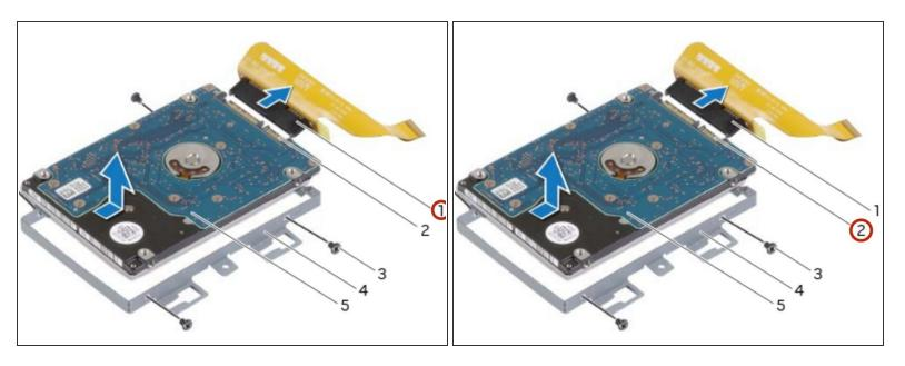
Disconnect the interposer from the secondary hard-drive connector.
