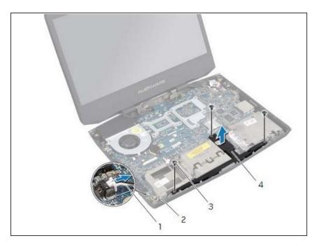
Replace the screws that secure the subwoofer to the computer base.
