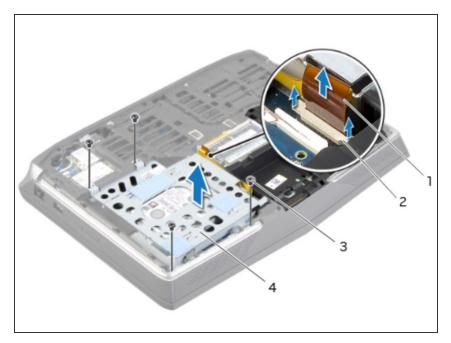
Replace the screws that secure the secondary hard-drive to the secondary hard-drive bracket.
