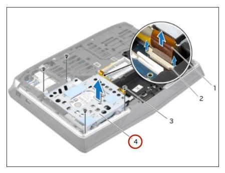
Lift the secondary hard-drive assembly off the computer base.
