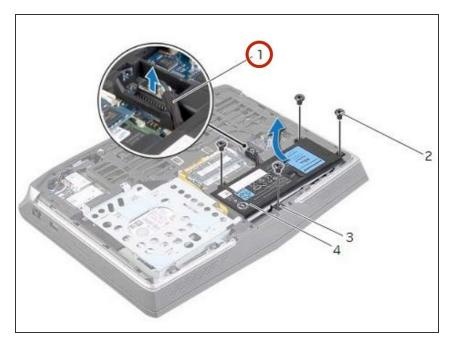
Using the battery cable, lift the battery and release it from the tabs on the computer base.
