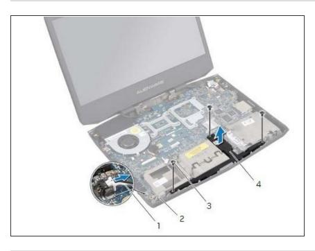
Route the subwoofer cable through the routing guide and connect the cable to the system-board connector.
