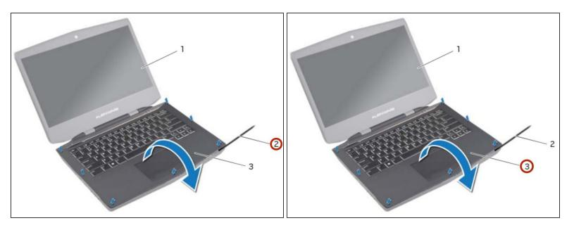
Using a plastic scribe, pry the palm-rest assembly from the computer base.
