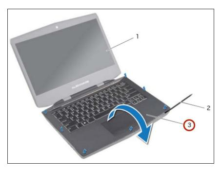
Carefully lift the palm-rest assembly and turn it over.
