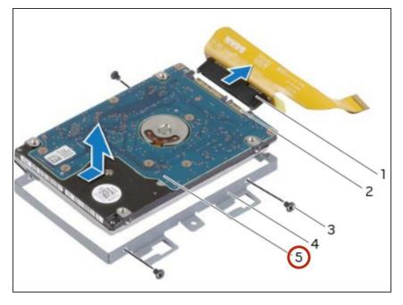
Connect the interposer to the secondary hard-drive connector.
