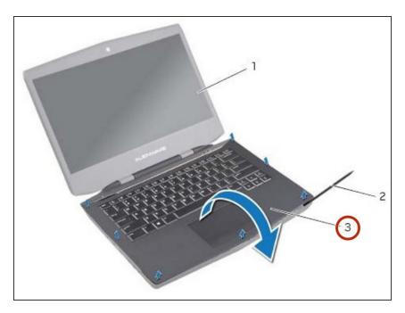
Turn the **NEW** palm-rest assembly over and slide the status-light board cable through the slot on the computer base.
