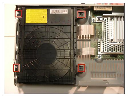
To remove the disc hub all you have to do is remove the 4 screws holding it down.
