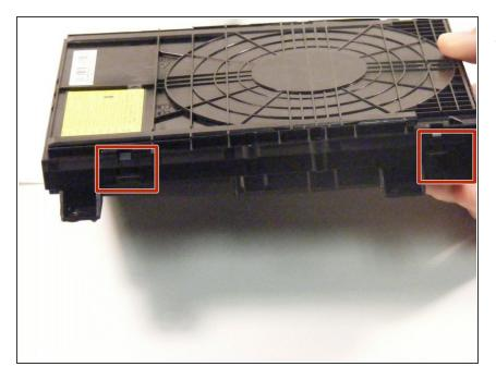
To replace the disc tray open the disk hub and unsnap the sides of the device.
