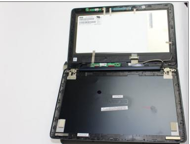
After removing the screws, use the metal spudger to gentle pry open the screen casing from the flip book casing.
