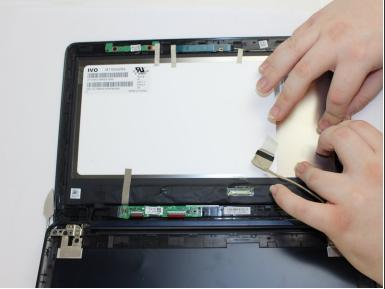
Gently remove all the connections and tape you see attached to the screen with tweezers.
