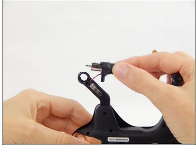
Hold the base of the arm while gently pulling the motor cover away from the arm.
