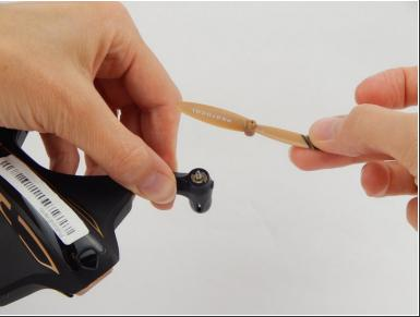
• Use a moderate amount of force to pry the propeller out of its base. The propeller should pop off.
