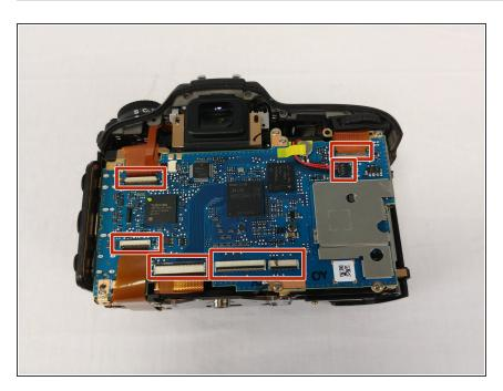
Disconnect the LCD ribbon cables and power cable from the motherboard.
