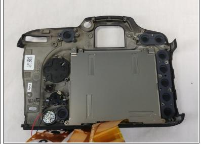
• Unscrew all 16 screws around the back plate of the camera.
