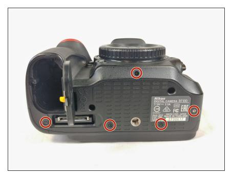
Remove the five screws on the bottom of the camera with a JIS #000 head screwdriver.
