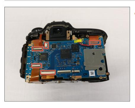
Undo the 5 ribbon cable connectors by flipping the latches up with a plastic spudger.
