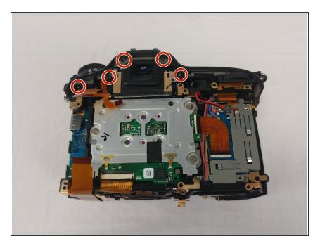
Remove these 5 screws along the top of camera body.
