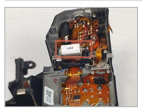
Remove the potentiometer and PCB off together.
