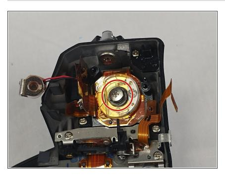
Remove the large screw in the middle of the dial-mode button. This allows you to replace it.
