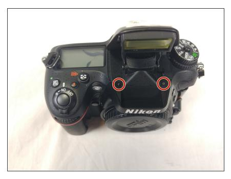
Remove these 2 screws on the top of the camera and pull the top screen, flash, and dial-mode button from the main body of the camera.
