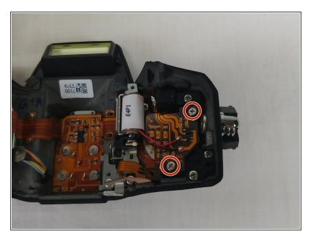
Remove the screws holding the dialmode PCB board down.
