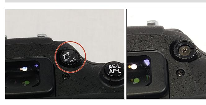
Remove the Diopter adjustment control sticker and remove the screw under it.
