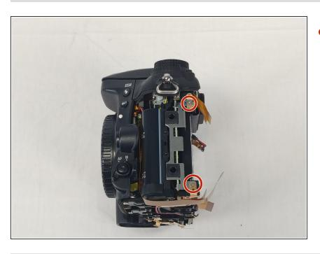
After following the guide to remove the back LCD screen from the motherboard, remove the 2 marked screws.
