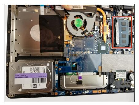
The RAM is a small rectangular component located on the opposite side of the lab top from where you pulled out the CD disc drive.
