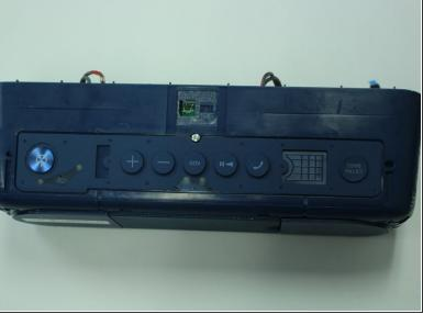
Remove the PH-1 (10mm) screw from the top of the speaker that is connected to the motherboard.
