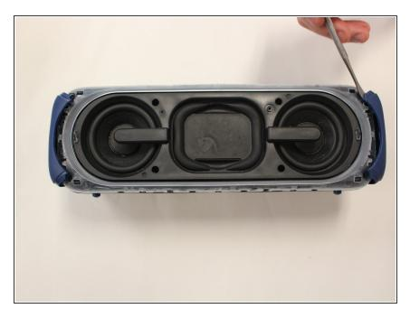
Pry the two remaining rubber pieces of the casing completely away from the body of the speaker with the same metal pry tool.
