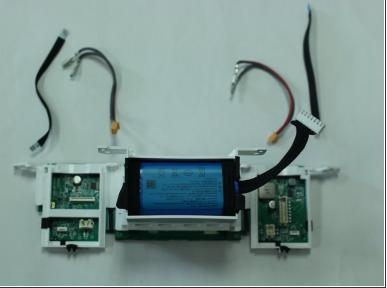
Remove the wires connected to the back of the motherboard before removing the white cover.
