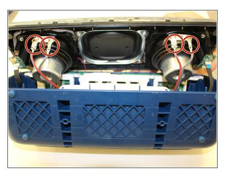
Once you have gotten to the internal parts of the speaker, there are seven wires connecting the speaker plate to the body of the speaker.
