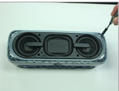
Once you have removed the outer blue casing, four T-8 screws (15 mm long) will be revealed on each corner. After removing these screws, simply pull the top part of the speaker way from the body to get the inner part of the speaker.
