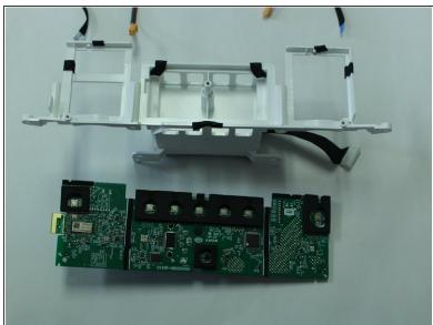
Remove the PH-1 screws (10 mm) from the motherboard to detach it from the outer white casing.
