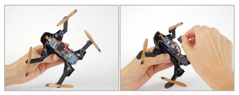
• Remove the foam adhesive pad located on the Wi-Fi transmitter board.
