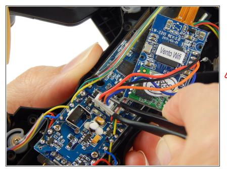
Disconnect the white clip that connects the four colored wires (black, orange, red, blue) to the motherboard.
