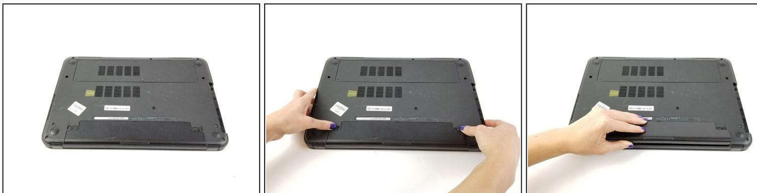
**⚠ Remove the battery to avoid electrical discharge while working with this system.**
