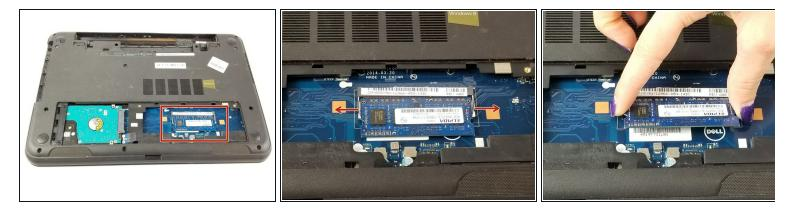
• Remove the memory card by pulling apart the latches holding it in place.
