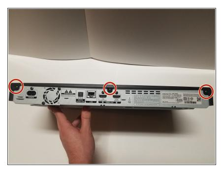
On the back side of the unit, remove the three 8.1mm screws marked with a Phillips #1 screwdriver.
