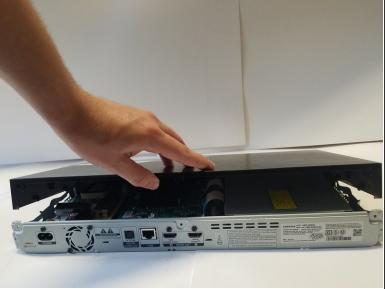
• From the back, lift the case upwards away from the unit then forwards, releasing the prongs on the front.
