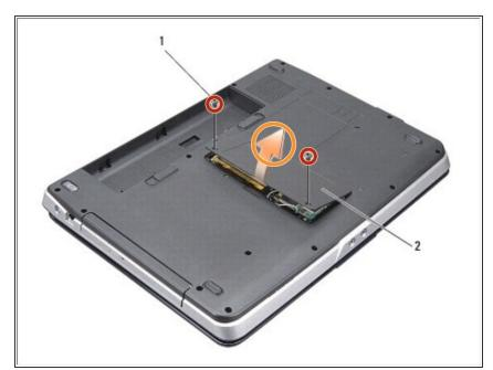
Remove the two screws from the module cover.
