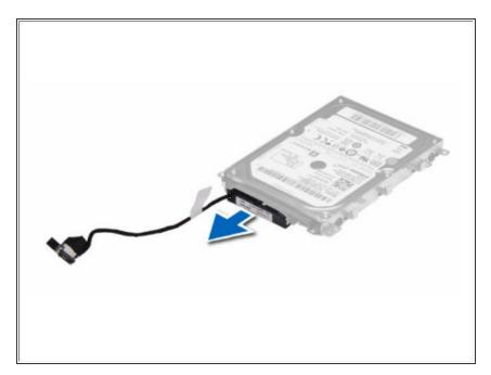
Disconnect the hard-drive connector from hard drive.
