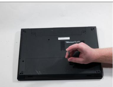
Using a #0 Phillips screwdriver, remove the 2.0mm screw from the back of the device beside the vents.
