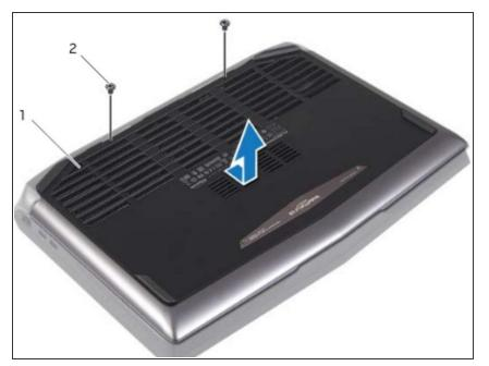
Align the tabs on the **new** base cover with the slots on the computer base
