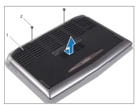
Slide the base cover toward the back of the computer and align the screws holes on the base cover with
