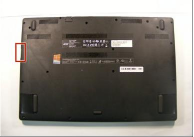
Use the spudger to remove the back plate in the highlighted area to carefully pop out the back plate.
