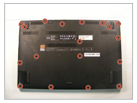
Use a Phillips #1 screwdriver to remove all eighteen 2.12 mm screws from the back plate of your Acer Aspire.
