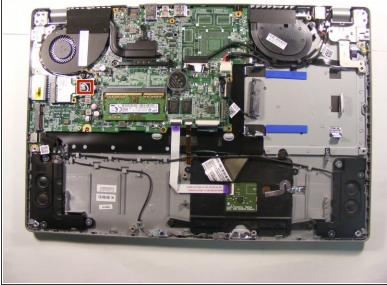
After the screws are removed, you will need to unplug it from the motherboard shown by the red
