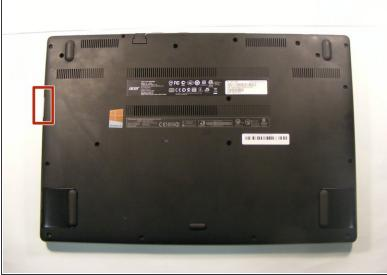
Use the spudger to slowly and gently work your away around the device, popping the bottom cover off the device.
