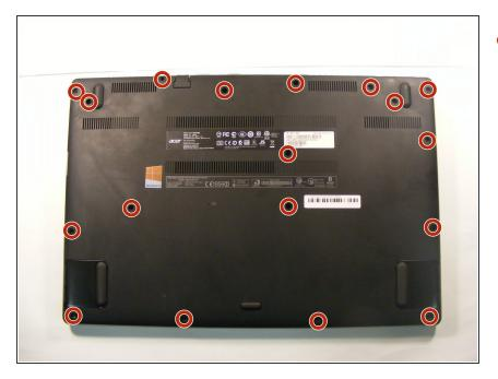
Remove all 18 of the marked screws (2.12 mm) using a Phillips #1 Screwdriver.
