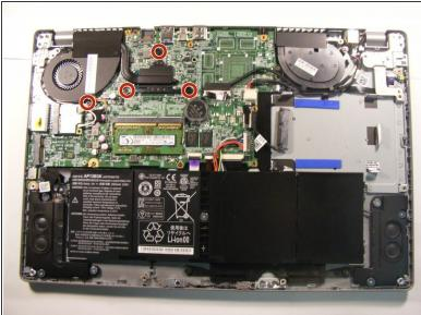
Remove the four marked screws (2.31mm) using a Phillips #1 Screwdriver.
