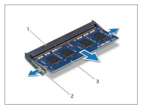
Slide the memory module firmly into the connector at a 45-degree angle and press the memory module down until it clicks into place. If you do not hear the click, remove the memory module and reinstall it.
