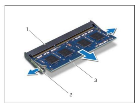
Align the notch on the NEW memory module with the tab on the memorymodule connector.
