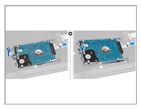
• Lift the hard drive to remove it from the computer [1,2].
