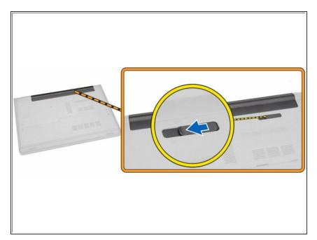
Slide the release latch outwards to unlock the battery.
