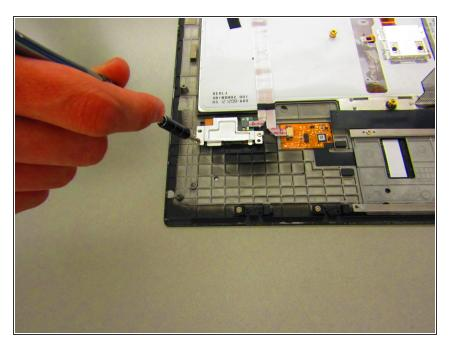
Locate the Fingerprint Reader and metal frame on the left side of the keyboard tray.
