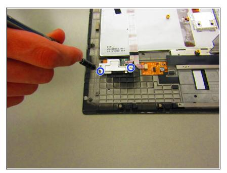
• Unscrew the two silver screws to remove the metal frame.
