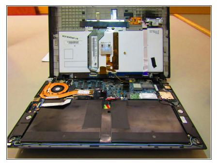
• Flip the device over and open it to lift the keyboard tray from the body of the device.
