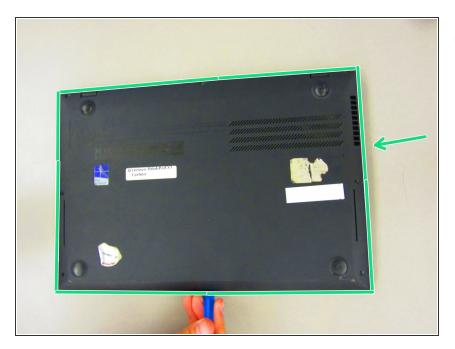
Slide the plastic opening tool along the edge of the device to separate the keyboard tray.
