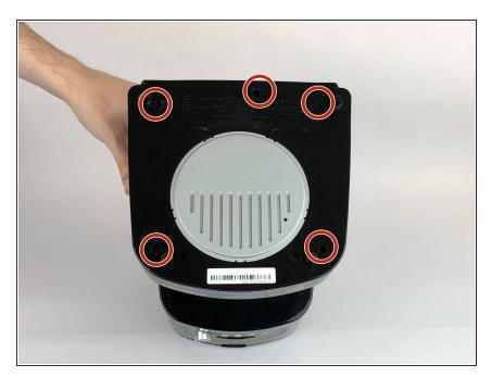
Remove the five 1.6mm Phillips #1 screws from the bottom panel.
