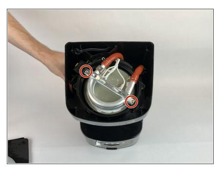
Remove the two 1.6mm Phillips #0 screws from the retaining bracket on the heating element.
