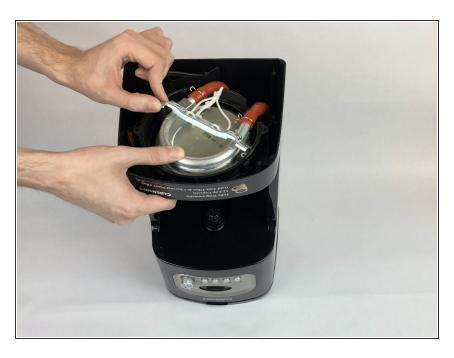
Remove the retaining bracket and allow it to hang off of the heating element.
