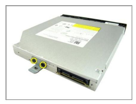
Remove the screws that secure the optical drive bracket.
