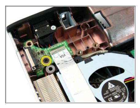
Remove the screw that secures the VGA board.
