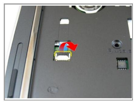
Release the latch on the system board connector and then disconnect the power button cable.
