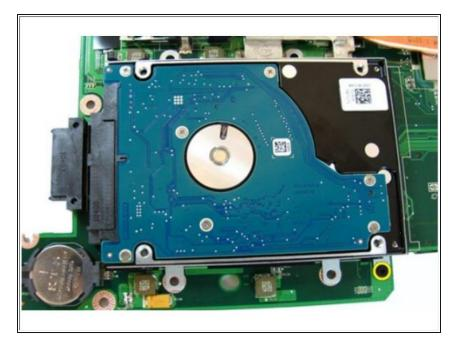
Remove the screws that secures the hard drive bracket
