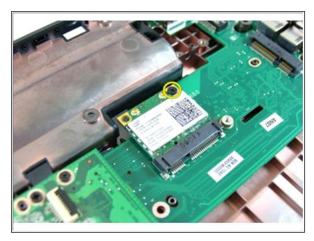
Remove the screw that secures the WLAN card.
