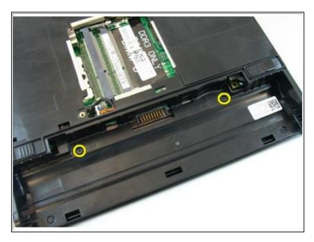
Remove the screws in the battery compartment.
