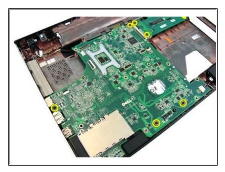
Remove the screws that secures the system board.
