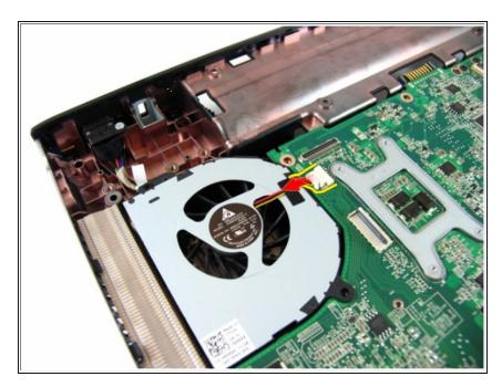
Disconnect the system fan cable from the system board.
