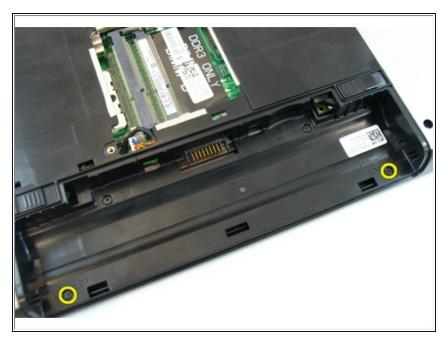
Remove the screws that secure the hinge cover.
