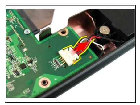
Disconnect the speaker cable from the system board.
