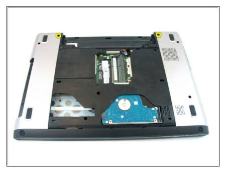
• Remove the screws that secure the display hinge.
