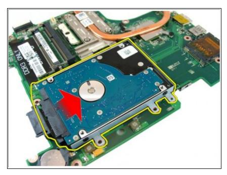
Slide the hard-drive module to release it from the system board
