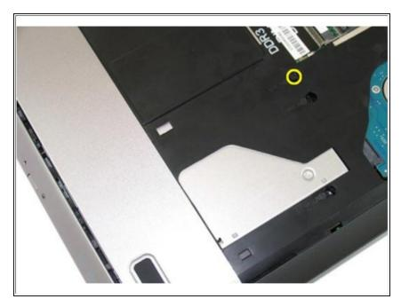
Remove the screw that secures the optical drive to the computer.
