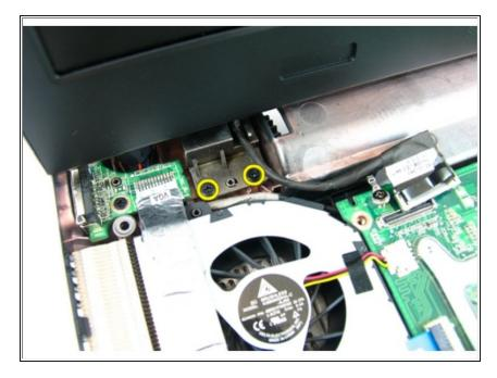
Remove the screws that secure the left hinge.
