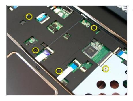
Flip the computer around and remove the screws that secures the palm rest.
