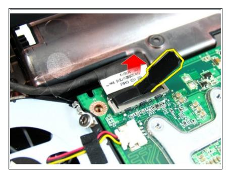
Disconnect the LVDS cable from the system board.
