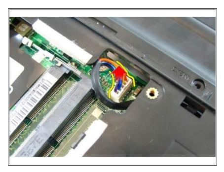
Disconnect the DC-in cable connector from the system board.
