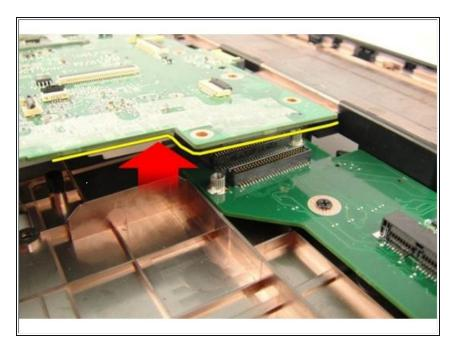
Disconnect the system board from the Input/Output panel.
