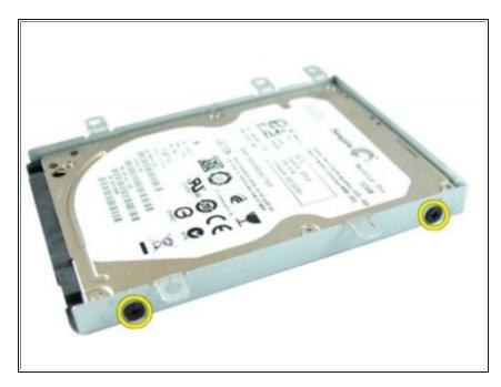
• Remove the screws that secures the hard-drive bracket on one side.
