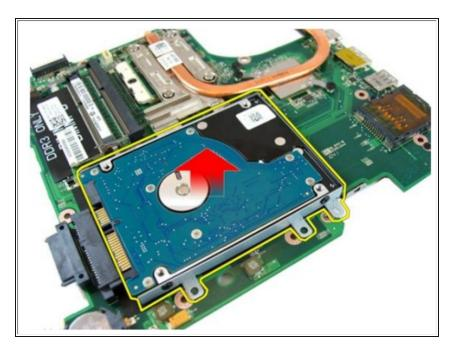
Remove the hard drive module from the system board.
