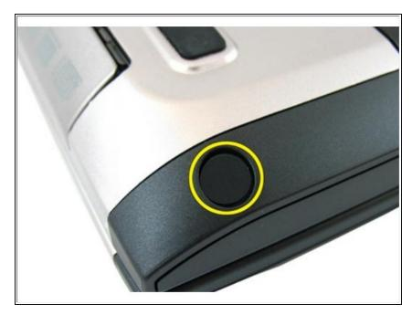
• Remove the rubber from the bottom base on the right side.
