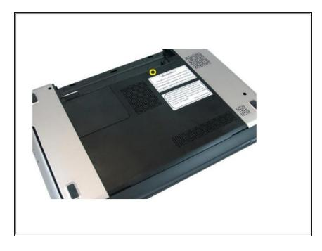
Loosen the screw that secures the memory door.
