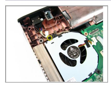
Remove the screw that secures the system fan.
