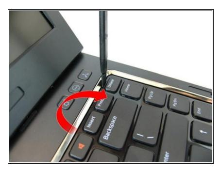
Press the keyboard down. Pry the keyboard with the use of a flat-head screwdriver towards the display to reveal the first keyboard retainer.
