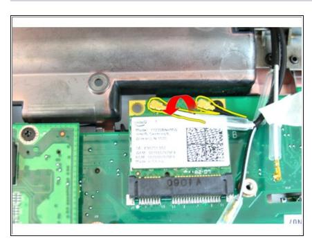
Disconnect the wireless local area network (WLAN) antenna cable.
