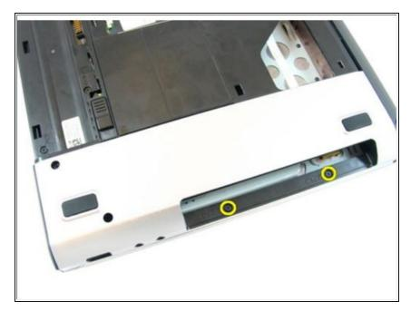
Remove the screws in the optical drive compartment.
