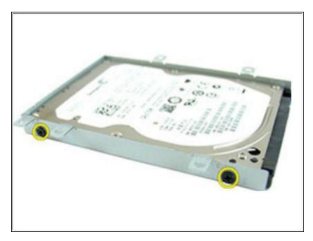
Remove the screws that secures the hard-drive bracket on the other side
