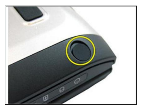
Remove the rubber from the bottom base on the left side.
