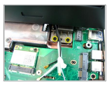
• Remove the screws that secure the right hinge.
